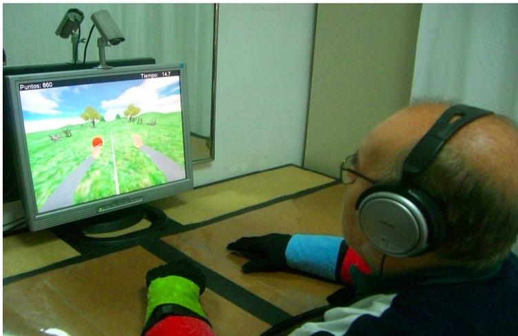
The Rehabilitation Gaming System (RGS) is a Virtual Reality (VR) based system for the rehabilitation of the motor deficits of the upper extremities. During the training, the movements of the user are mimicked by two virtual arms embedded within a virtual world. This results in simultaneous action execution and observation. We hypothesize that such a scenario may enhance and/or speed-up recovery after a brain lesion.
